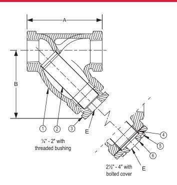
Style B Y-Strainer, Class 250 NPT Cast Iron (ASTM A 126, Class B)
