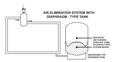
The third essential component in the air elimination system is the tangential-type air separator which separates entrained air from flowing system water by the creation of a vortex which will allow free air to rise in the center, the point of lowest velocity, to the air collection chamber in the body of the air elimination valve.
