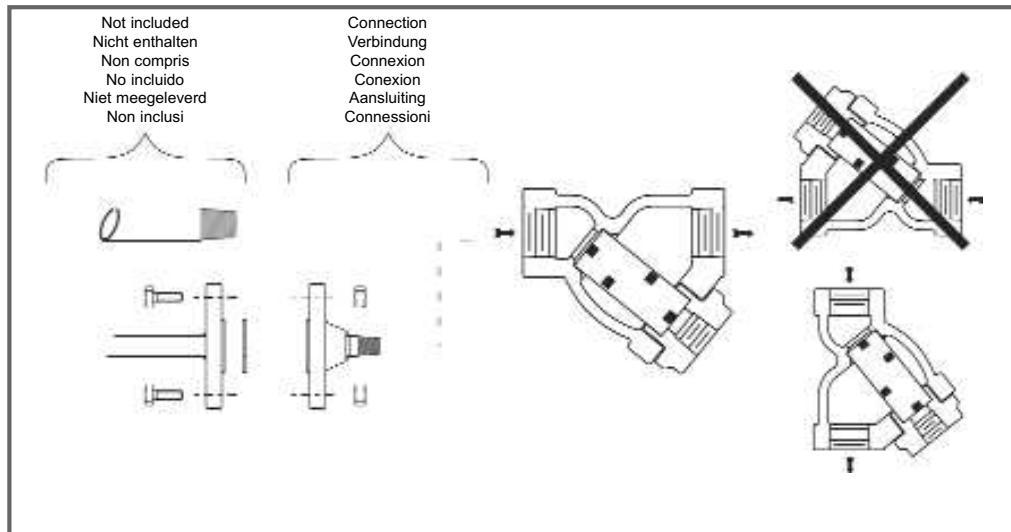
**STANDARD BLOW-DOWN IS OPEN. MAKE SURE TO SCREW PLUG OR VALVE IN IT!**
