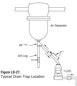
Drain traps dispose of water that collects in many places in a compressed air system. Each drain trap arrangement must be considered individually.
